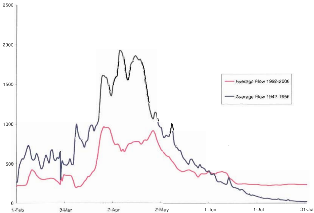
Figure 7-4. Average annual springtime and summer flow at the Bowman Dam for the periods 1942-1956 and 1992-2006.
